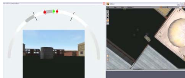
Figure 2. Illustration of asymmetry in the vehicle width indicator due to the left object (barrel) being closer to the vehicle as compared to the right object (distant wall).
