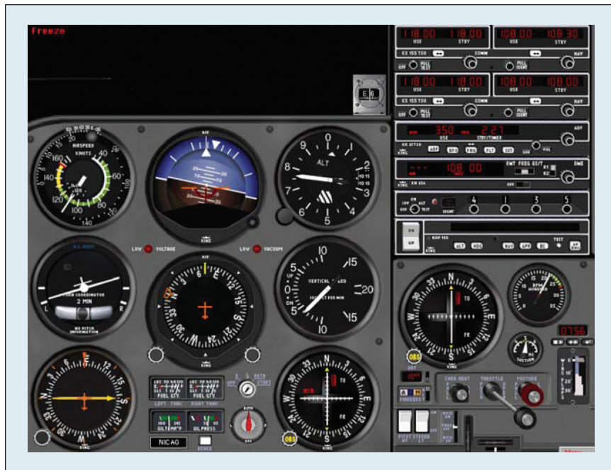
Figure 1. An emulation of a traditional dials-based cockpit display.
